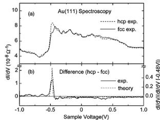
Au surface state at -0.5 V at 4 K in UHV
